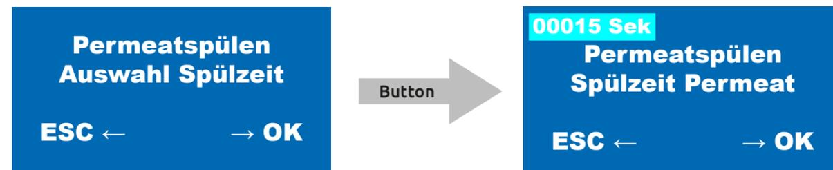
The time will now flash and can be changed between 15 and 300 seconds with the (+) or (-) key. Less than 15 seconds is not available to protect the system from possible damage. Confirm the selection with the **OK-Key**.
