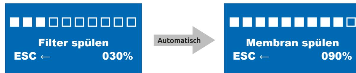
While rinsing the membranes (Membran spülen), the disinfectant is removed from the membrane and drains into the wastewater tube connection.
