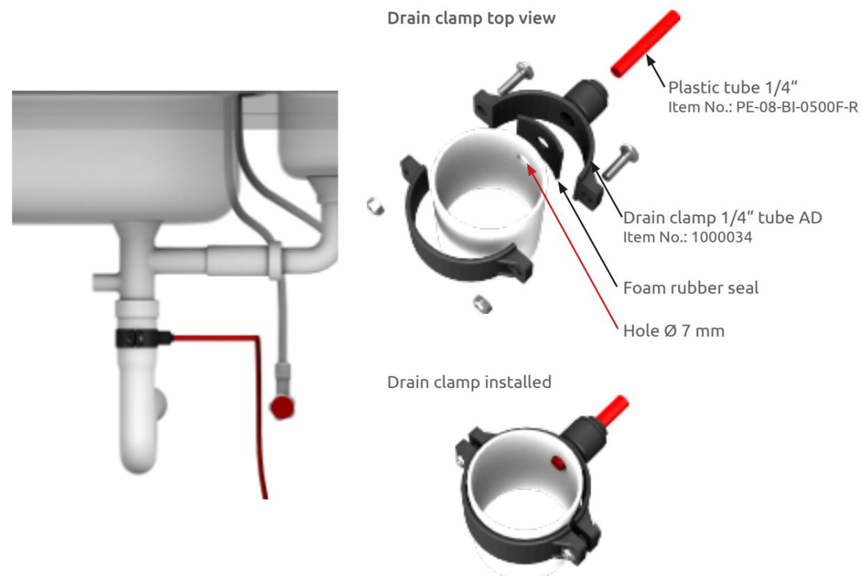
**i** Install the drain clamp above the odour trap of the siphon.
