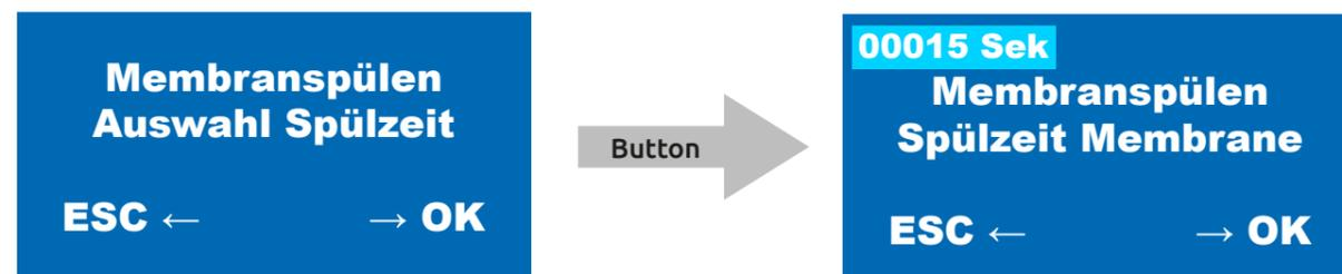
The time will now flash and can be changed between 15 and 300 seconds with the (+) or (-) key. Less than 15 seconds is not available to protect the system from possible damage. Confirm the selection then with the **OK-Key**.
