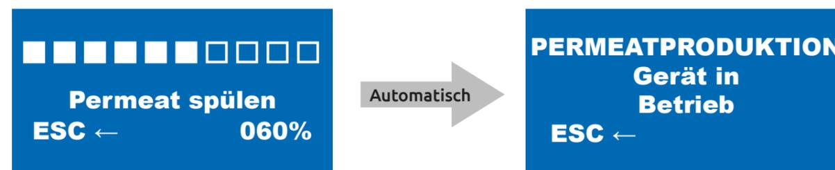
When the commissioning program (IB-Programm) is completed, and the withdrawal tap is open, the Verdanium Home changes automatically to permeate production (Permeatproduktion). Continue operating the Verdanium Home for additional 7 - 10 minutes to flush out any remaining disinfectant residues, and check that all connections are leak-proof.
