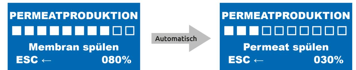
After rinsing, the Verdanium Geo automatically changes to ultra-pure water production. The following messages appear on its display:
