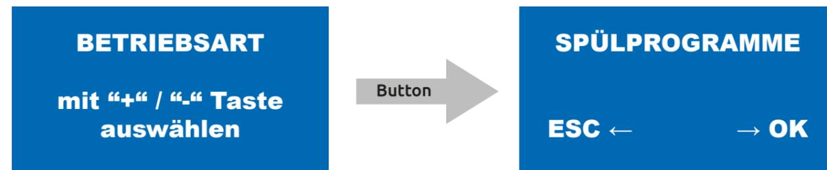
After you have selected the rinsing programs with the **OK key**, you can choose and manually set the rinsing time of the permeate rinsing. The rinsing time is shown at the top left of the display. Press the **OK-Key** once to select the time.
