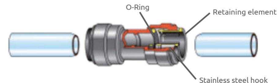
The John Guest connector consists of the connector body, retaining elements with a stainless-steel hook and NBR-O-Rings for sealing. The connector can be assembled or disassembled without using tools. The connection is solid before it seals watertight!
