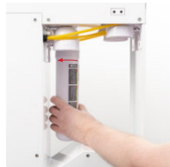
Turn the second filter cartridge counterclockwise 90° out of the filter head to change the second filter cartridge.
