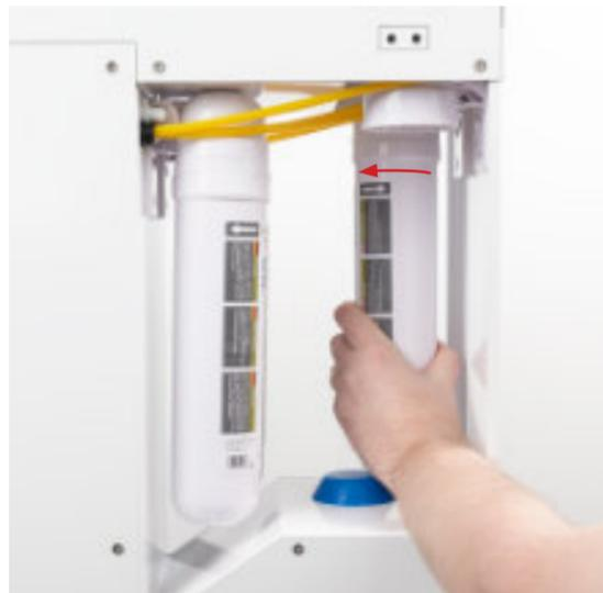
Turn the second pre-filter cartridge counterclockwise 90° out of the filter head to change the second pre-filter cartridge.
