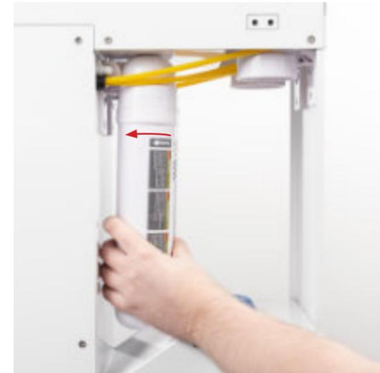
Change the post-filter cartridges in the same way as the pre-filters. Turn filter cartridges counterclockwise by 90° out of the filter head to change the filter cartridge.
