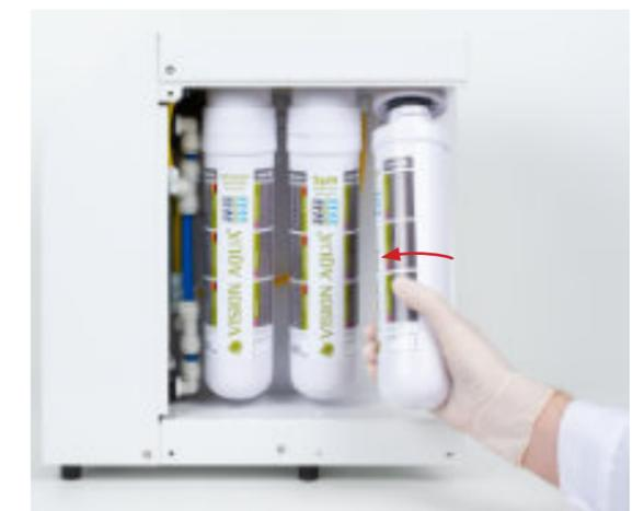
Turn pre-filter cartridge counterclockwise 90° out of the filter head to change the filter unit.
