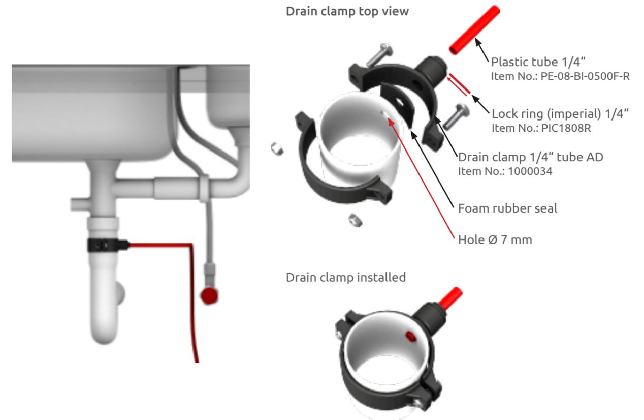
Install the drain clamp above the odour trap of the siphon.
