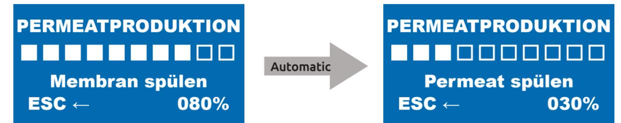
After rinsing, the Verdanium HOME automatically changes to ultra-pure water production. The following messages appear on its display:
