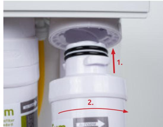
Press the new filter cartridges into the filter heads of the Verdanium HOME and turn them 90° clockwise.
