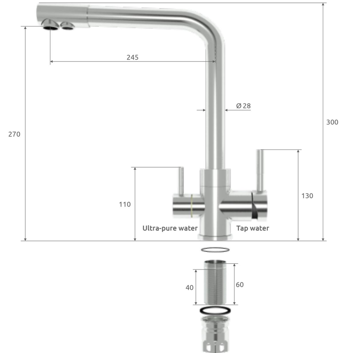
Both connections to the angle valve and the Verdanium HOME are under full water pressure and should be installed with particular care. Check that both connections, with the angle valve opened, are leak-proof.
