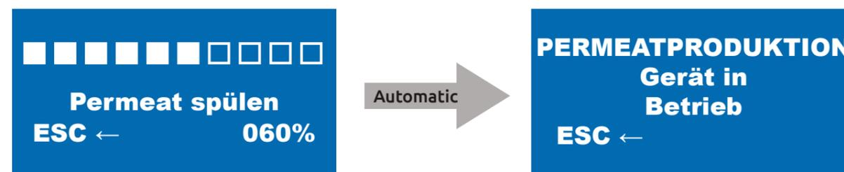
When the IB-Programm is completed, and the extraction tap is open, the Verdanium HOME changes automatically to permeate production. The Verdanium HOME is now ready for use.
