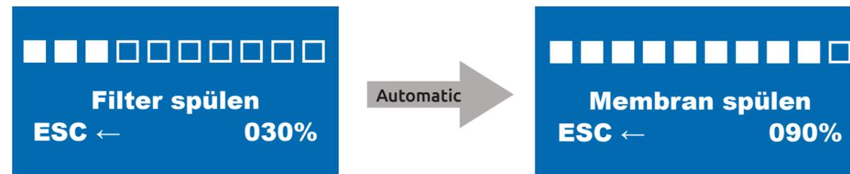
When rinsing the membranes (Membran spülen), the disinfectant is removed from the membrane and drains into the waste-water connection.
