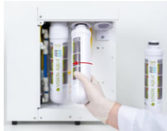
Turn pre-filter cartridge counterclockwise 90° out of the filter head to change the second PP filter unit.
