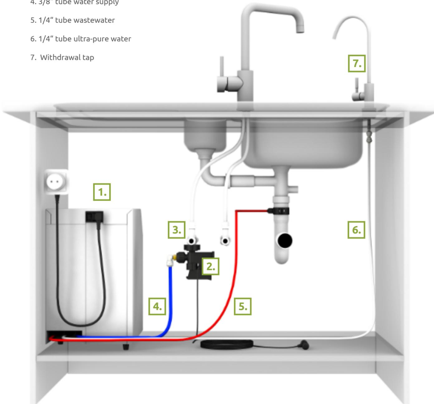
**The maximum tube length for the 1/4" pure water tube is 2 meters. For the 1/4" wastewater tube, the maximum tube length is 3 meters. Anything exceeding these limits must be adapted to a 3/8" tube.**
