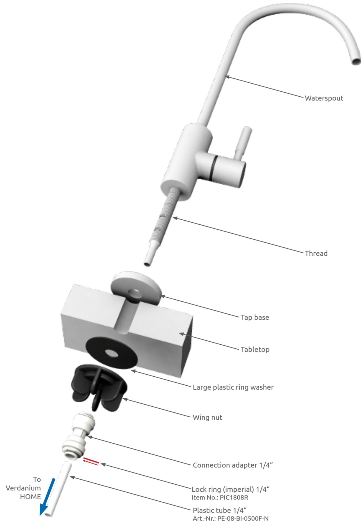
Ultra-pure water and tap water share a faucet, with the internal pipelines being separated from each other. This allows you to use your tap water as usual for washing, while at the same time, you have the option to obtain absolutely pure drinking water directly from one faucet.
